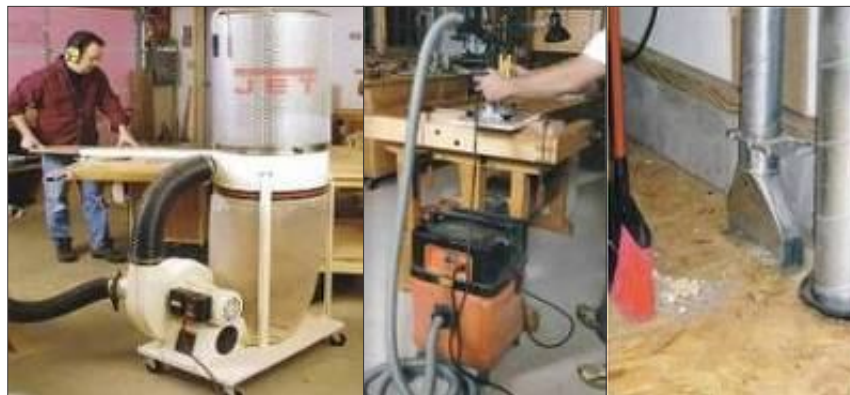
Figure 4. Central portable vacuum system (left), portable vacuum (middle), stationary vacuum system (right).
