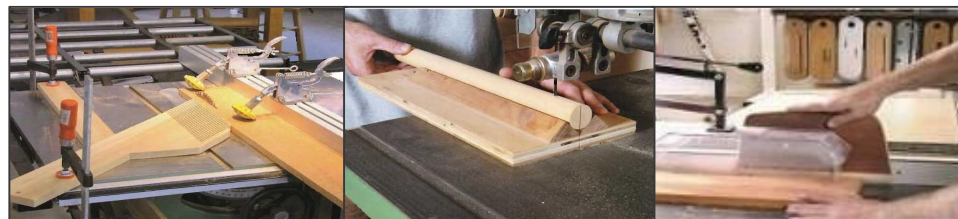
Figure 6. An arm for holding big pieces on the cutting table (left), a V-shaped device for cutting small pieces (middle), a device for more safety and ease in cutting (right).
